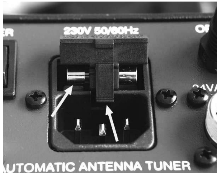
Fig. 5-1 Pulling out the AC line fuse.
