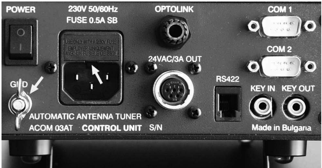
Fig.2-7 RCU rear panel, grounding terminal, and mains fuse.
